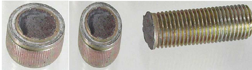
Figure 1: Typical Fastener Failure by Hydrogen Embrittlement
